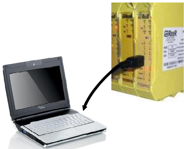
Figure 2 - USB 2.0 front panel connector
